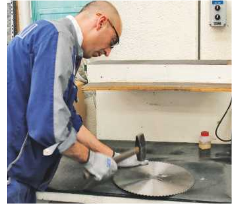
The skill of the workforce then comes into play by tapping the blade to address any irregularity
